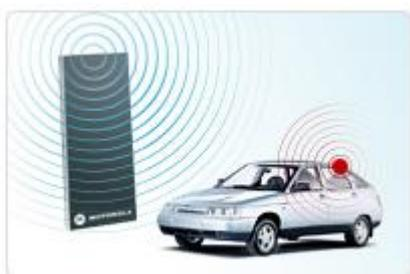
The RFID (radio frequency identification) enables using radio waves for automatic identification of transport objects. For this purpose, special programmable tags are fixed on the objects (in our case — motor vehicles), which are identified by RFID-readers at a distance of 5–8 meters.
