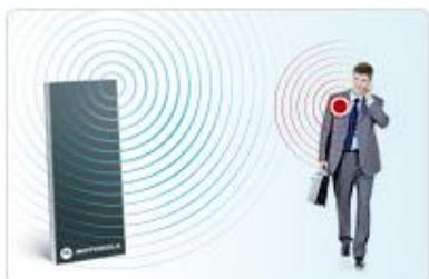
Radio frequency identification is based on the use of radio waves to capture and read information with a special mark on the badge or bracelet of a visitor. When it passes through a checkpoint, RFID-tag read by the antenna, the signal goes to the RFID-reader, and then - on the database server that stores all the information for all visitors.
