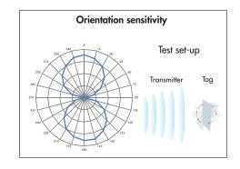
All the graphs are indicative: performance in real life applications may vary. The data has been determined based on calculations for transmitters with a 2W ERP output power level.
