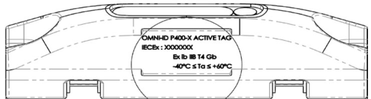
IECEx Laser Marking on the side of the tag
